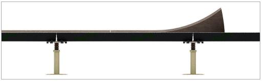
PVC tiles have a different size compared to the raised floor panels. This means that the PVC tiles cover the seams of the raised floor
